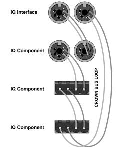
Fig. 3.10 Crown Bus Wiring "Loops" from the Output to the Input of Each IQ Component
